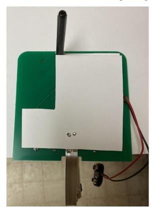
Put another lock washer on each of the 3/8-inch bolts of the upper half of the key; put the holes in the cardboard backing through the bolts and secure with a second pair of nuts. Use the needle nose pliers to tighten the nuts, using the screwdriver to hold the bolts in place. At this point, the bolts should not be able to move; if they do, retighten the first nut.
